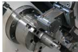
Chuck Air Blow (Upper Chuck)
