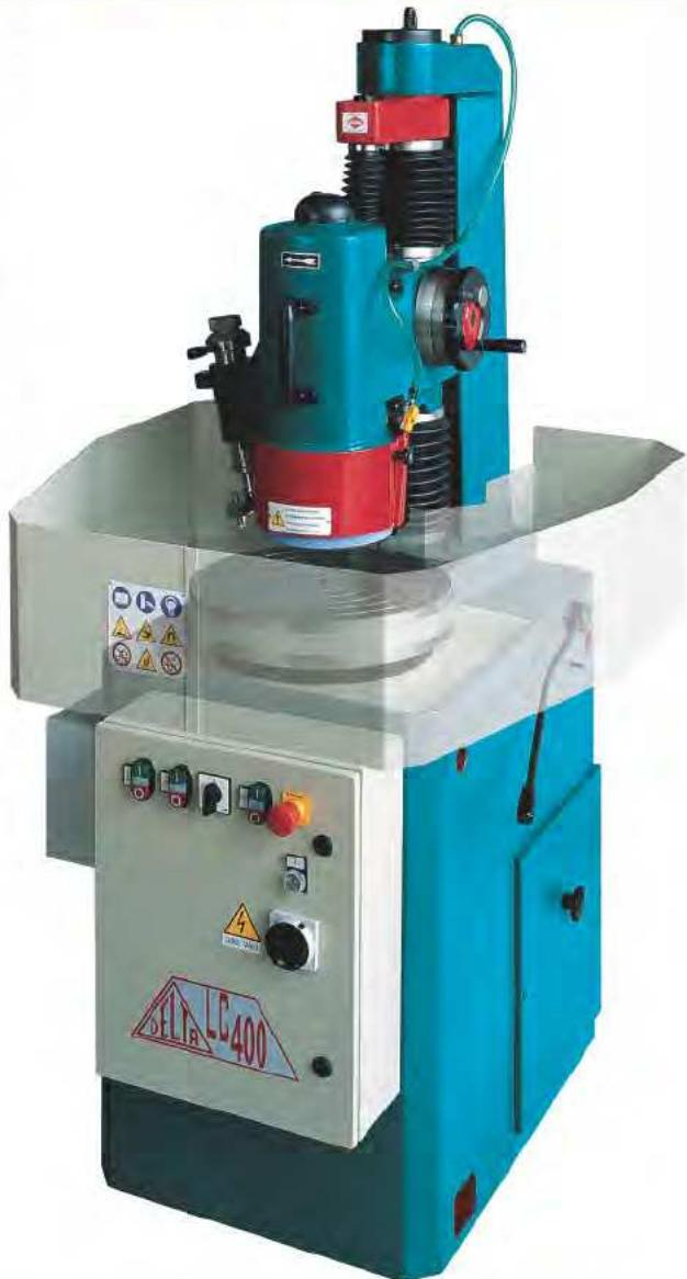
an electronic speed variator, which allows stepless variations from 3 to 30 rpm; a digital display shows the set speed immediately.
