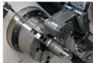
Chuck Air Blow (Upper Chuck)
