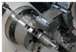
Chuck Air Blow (Upper Chuck)
