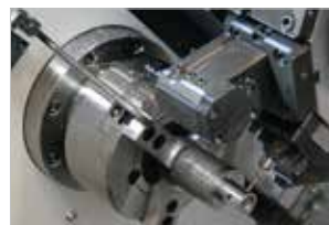
Chuck Air Blow (Upper Chuck)
