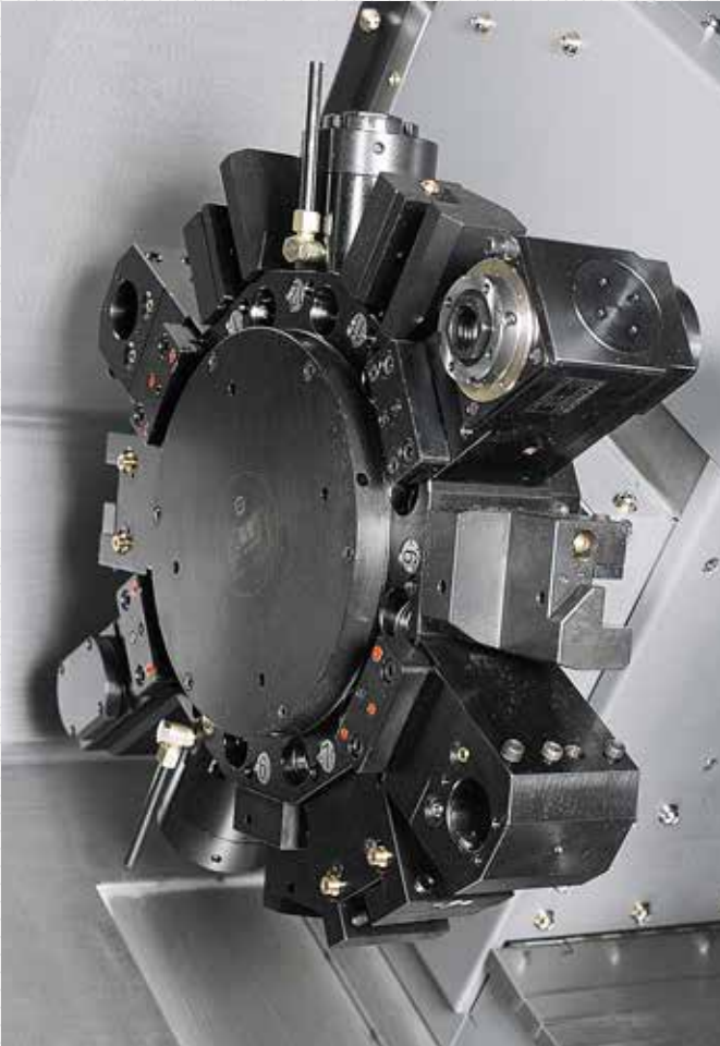
The 12 station VDI turret is designed with 3 piece curvic couplings to reduce vibration during heavy duty cutting, which lengthens tool life.
