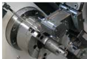
Chuck Air Blow (Upper Chuck)
